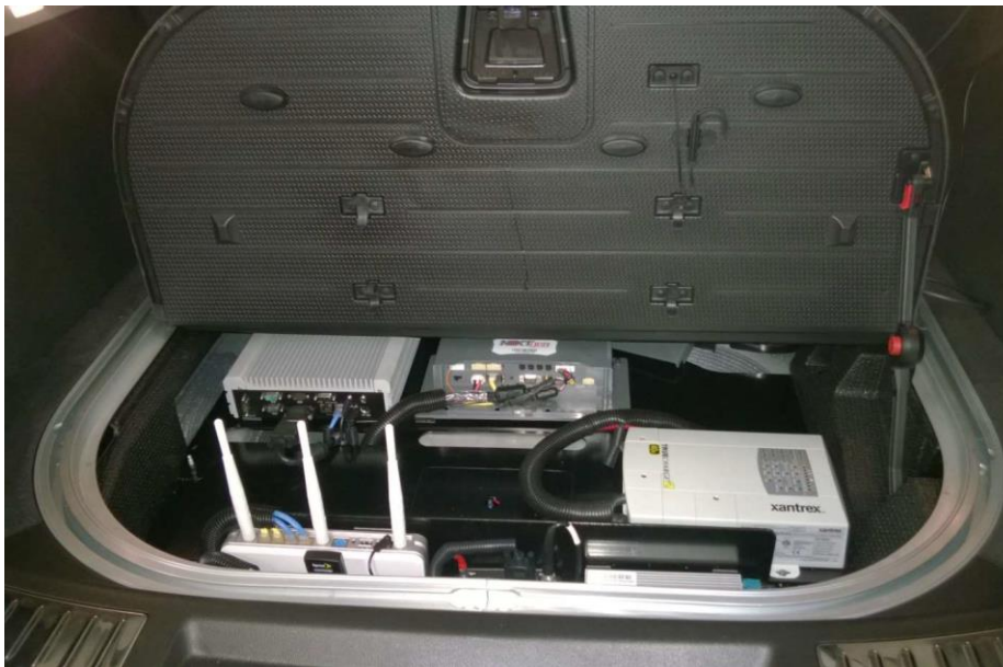
Figure 15. FHWA connected vehicle on-board equipment Source: Scott Washburn
