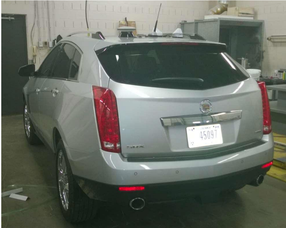
Figure 14. FHWA connected vehicle with equipment attached to the roof Source: Scott Washburn
