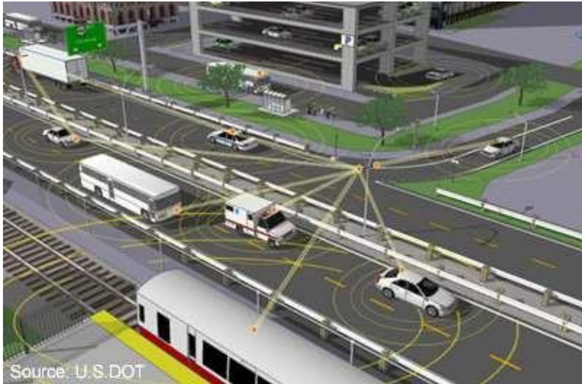
Figure 16. V2V and V2I technology between all modes of transportation
