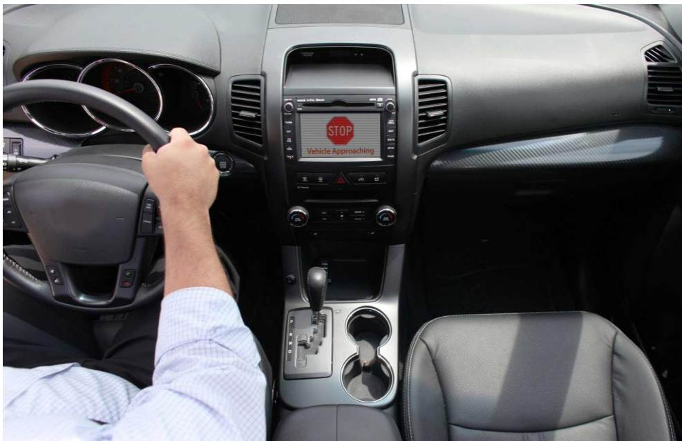
Figure 10. Implementation of driver warning message Source: USDOT
